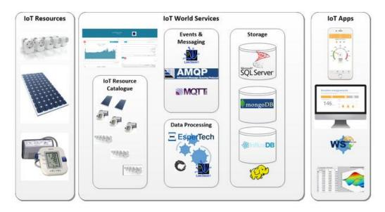
Figure 13: Medical device connectivity interface based on LinkSmart
