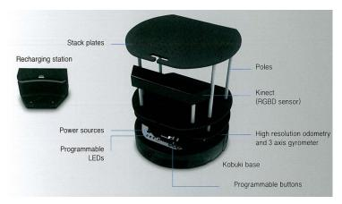
Figure 19. Components of the Turtlebot telepresence paltform.
