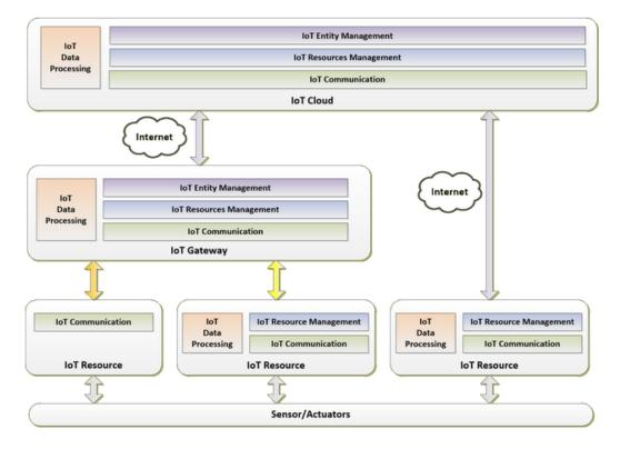
Figure 14: LinkSmart.net gateway & mechanism
