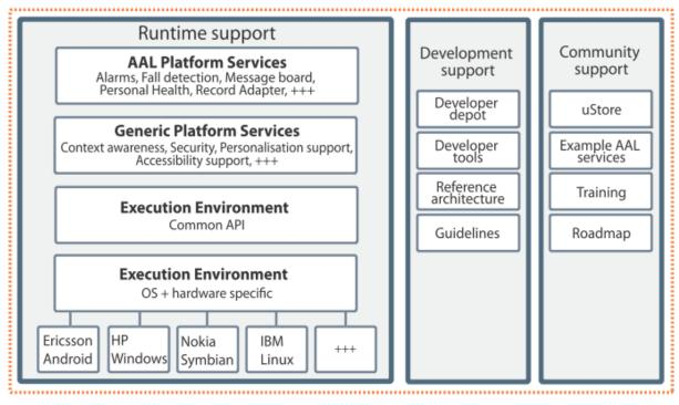
Figure 15. The universAAL platform architecture.
