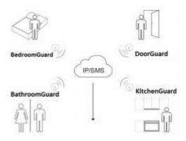
• KitchenGuard: Multiple sensors are set up in different places of the kitchen, monitoring the heat, smoke, and turning off the oven if a fall is detected upon it. A fixed time can be monitored too in order to prevent the stove to be used for more than a maximum desired time assigned by the user or the care taker.
