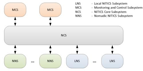
Figure 37: NITICS hardware architecture
