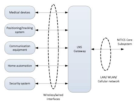
Figure 40: Local NITICS Subsystem functional architecture
