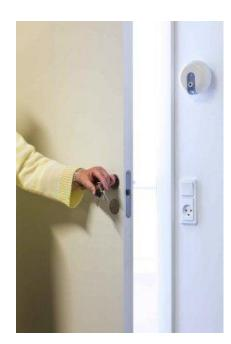
• BathroomGuard: Motion sensors are placed over the bathroom, they are capable of interacting with each other, detecting if the patient has reached the door, the sink, or the bathtub. If no movement is detected inside the bathroom for an specific interval of time, an alarm is triggered.
