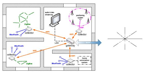
Figure 39: Communications between NITICS platform devices at the elderly home
